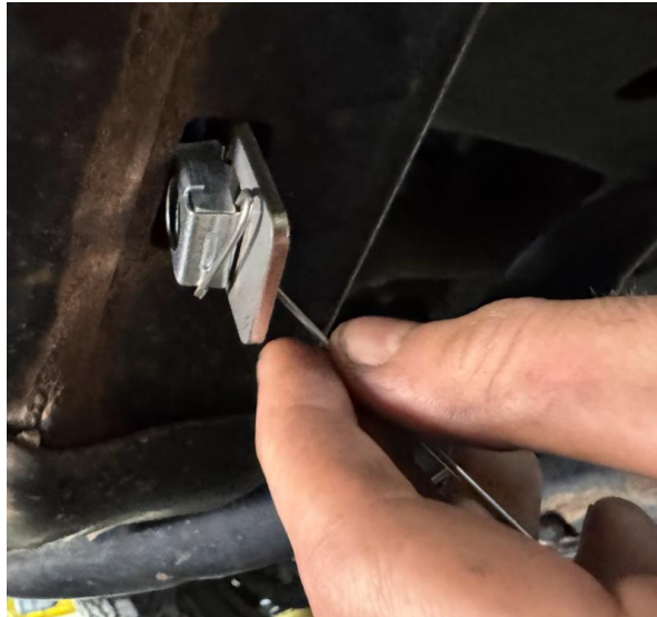
A Insert the plate into the square opening. B Rest the rod along the lower edge.
