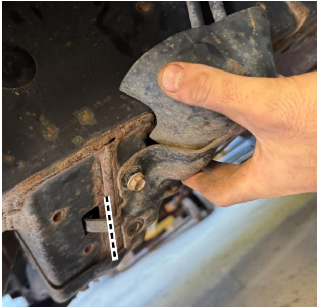
A Cover tab to trim or bend. B Clearance with the cover removed.
