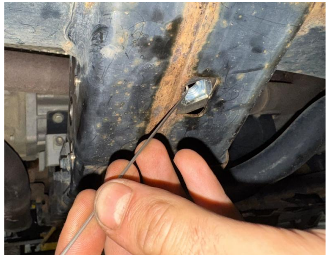
A Insert the plate into the square opening. B Rest the rod along the lower edge.
